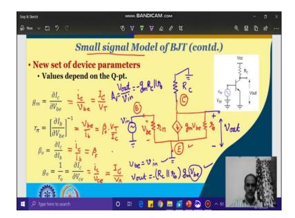
Now here we do have the small signal equivalent circuit of the BJT and let us try to see that how it can be utilized to get the gain of the circuit. So, along with the small signal equivalent circuit of the BJT let you also integrate the other components of the circuit.
