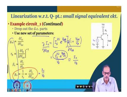
We have to take the expression of the collector current  $I_c$  which is having  $I_S^{(C)}$   $e^{\frac{V_{be}}{V_T}} \times \left(1 + \frac{V_{ce}}{V_A}\right)$ .
