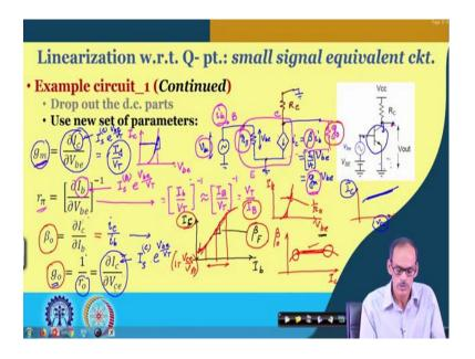
So, we are discussing that small signal equivalent circuit with respect to operating point which is basically linearization and we are talking about how do we. Once we have the circuit how we do linearize the circuit and so. So, whenever we are considering the equivalent small signal equivalent circuit, if I quickly draw the circuit we do have the small signal input and then base to emitter.
