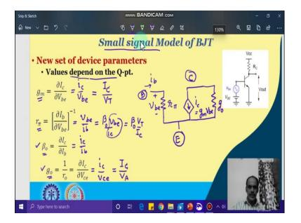
We understand from our previous discussion that, whenever we are linearizing a non-linear circuit, we are essentially drawing small signal equivalent circuit. And while you are drawing the small signal equivalent circuit of an amplifier we are replacing BJT by its small signal equivalent model and this model involves a certain set of parameter device, we call it is device parameters.
